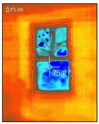
Commercially selling for only \$250, the FLIR One<sup>TM</sup> camera module provides its own power and is recharged separately, so it does not drain power from the cell phone. The  $160 \times 120$  pixel resolution imagery tracks surface temperatures from  $-20^{\circ}$  C to  $120^{\circ}$  C ( $-4^{\circ}$ F to  $248^{\circ}$ F), and it
